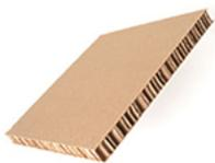
**Honeycomb Pads:** Provide superior cushioning, and protection for items up to 1,135 kg (2,500 lb). Made of recycled Kraft paper, they are an environmentally friendly alternative to bubble, foam or wood. Easily cut with a knife. Light weight makes them the perfect choice when trying to cut shipping costs. Ideal for void filling, blocking, bracing and layering, computer components, pre-assembled products with moving parts, and furniture.
